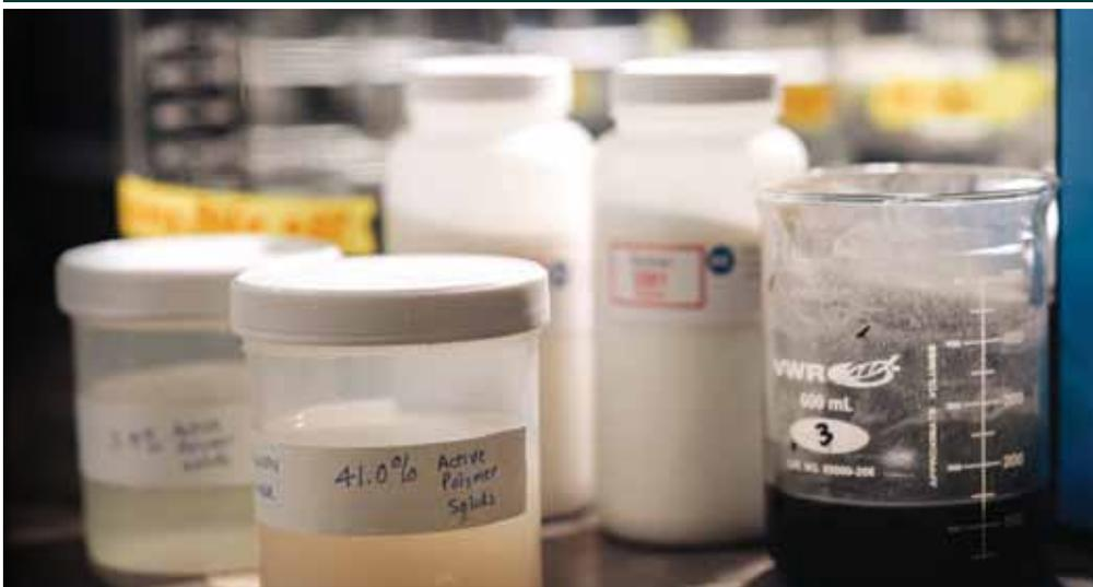
Sample emulsion and dry polymers that are used for sludge dewatering.
