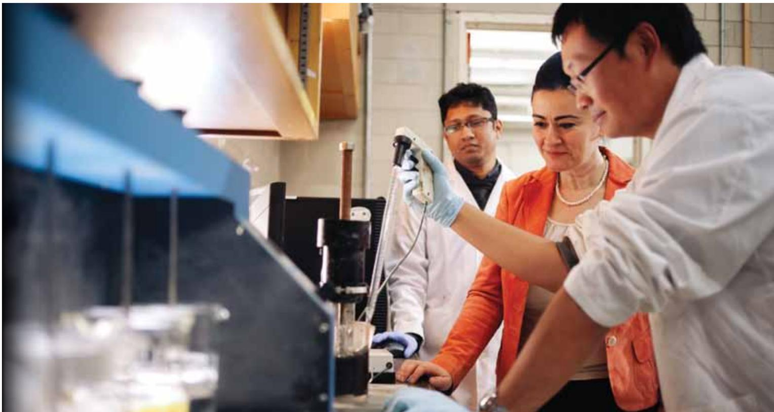
MASc candidate Yan Ze injects polymer in sludge before measuring its rheological properties to predict its behaviour during dewatering.
