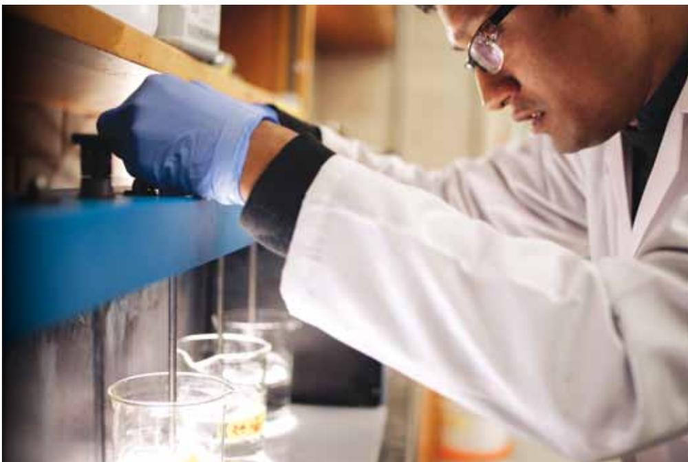
PhD candidate Muhammad Salam conducting a jar test experiment to determine the optimum polymer dose of sludge samples.
